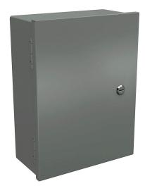
Wiegmann enclosure, NEMA 1, 16 x 12 x 6in (HxWxD), wall mount, carbon steel, ANSI 61 gray, powder coat finish, single-door, 1/4-turn flush-mounted latch.
