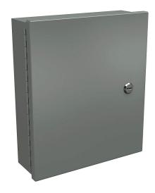
Wiegmann enclosure, NEMA 1, 14 x 12 x 4in (HxWxD), wall mount, carbon steel, ANSI 61 gray, powder coat finish, single-door, 1/4-turn flush-mounted latch.
