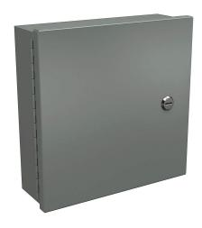
Wiegmann enclosure, NEMA 1, 12 x 12 x 4in (HxWxD), wall mount, carbon steel, ANSI 61 gray, powder coat finish, single-door, 1/4-turn flush-mounted latch.
