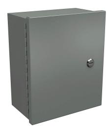
Wiegmann enclosure, NEMA 1, 12 x 10 x 6in (HxWxD), wall mount, carbon steel, ANSI 61 gray, powder coat finish, single-door, 1/4-turn flush-mounted latch.
