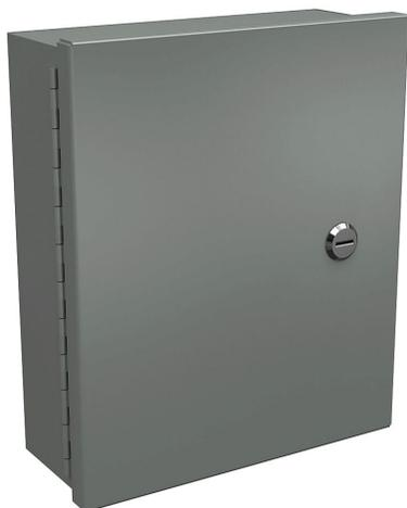
Wiegmann enclosure, NEMA 1, 12 x 10 x 4in (HxWxD), wall mount, carbon steel, ANSI 61 gray, powder coat finish, single-door, 1/4-turn flush-mounted latch.
