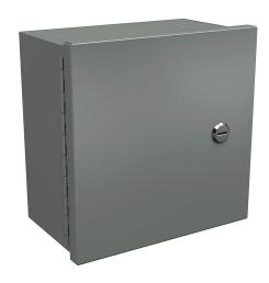
Wiegmann enclosure, NEMA 1, 10 x 10 x 6in (HxWxD), wall mount, carbon steel, ANSI 61 gray, powder coat finish, single-door, 1/4-turn flush-mounted latch.
