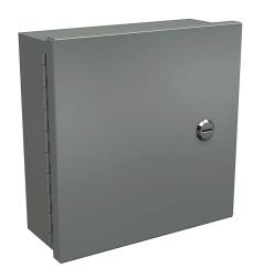
Wiegmann enclosure, NEMA 1, 10 x 10 x 4in (HxWxD), wall mount, carbon steel, ANSI 61 gray, powder coat finish, single-door, 1/4-turn flush-mounted latch.
