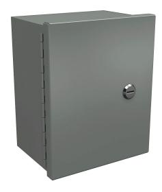
Wiegmann enclosure, NEMA 1,  $10 \times 8 \times 6$  in (HxWxD), wall mount, carbon steel, ANSI 61 gray, powder coat finish, single-door, 1/4-turn flush-mounted latch.
