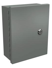
Wiegmann enclosure, NEMA 1, 10 x 8 x 4in (HxWxD), wall mount, carbon steel, ANSI 61 gray, powder coat finish, single-door, 1/4-turn flush-mounted latch.
