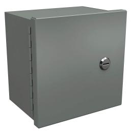
Wiegmann enclosure, NEMA 1, 8 x 8 x 6in (HxWxD), wall mount, carbon steel, ANSI 61 gray, powder coat finish, single-door, 1/4-turn flush-mounted latch.
