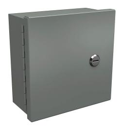
Wiegmann enclosure, NEMA 1, 8 x 8 x 4in (HxWxD), wall mount, carbon steel, ANSI 61 gray, powder coat finish, single-door, 1/4-turn flush-mounted latch.
