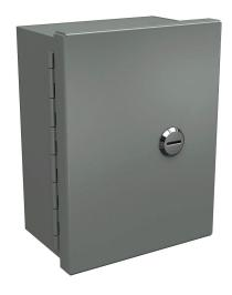
Wiegmann enclosure, NEMA 1, 8 x 6 x 4in (HxWxD), wall mount, carbon steel, ANSI 61 gray, powder coat finish, single-door, 1/4-turn flush-mounted latch.
