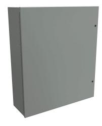
Hammond enclosure, NEMA 1, 42 x 36 x 12in (HxWxD), wall mount, carbon steel, ANSI 61 gray, powder coat finish, single-door, 1/4-turn semi-flush latch.
