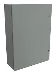
Hammond enclosure, NEMA 1, 42 x 30 x 12in (HxWxD), wall mount, carbon steel, ANSI 61 gray, powder coat finish, single-door, 1/4-turn semi-flush latch.
