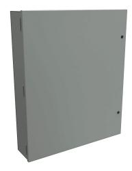
Hammond enclosure, NEMA 1, 36 x 30 x 7in (HxWxD), wall mount, carbon steel, ANSI 61 gray, powder coat finish, single-door, 1/4-turn semi-flush latch.
