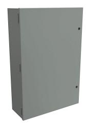
Hammond enclosure, NEMA 1, 36 x 24 x 9in (HxWxD), wall mount, carbon steel, ANSI 61 gray, powder coat finish, single-door, 1/4-turn semi-flush latch.
