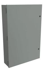
Hammond enclosure, NEMA 1, 36 x 24 x 7in (HxWxD), wall mount, carbon steel, ANSI 61 gray, powder coat finish, single-door, 1/4-turn semi-flush latch.
