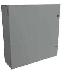
Hammond enclosure, NEMA 1, 30 x 30 x 9in (HxWxD), wall mount, carbon steel, ANSI 61 gray, powder coat finish, single-door, 1/4-turn semi-flush latch.
