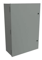
Hammond enclosure, NEMA 1, 30 x 20 x 9in (HxWxD), wall mount, carbon steel, ANSI 61 gray, powder coat finish, single-door, 1/4-turn semi-flush latch.
