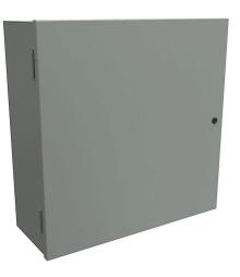
Hammond enclosure, NEMA 1, 24 x 24 x 9in (HxWxD), wall mount, carbon steel, ANSI 61 gray, powder coat finish, single-door, 1/4-turn semi-flush latch.
