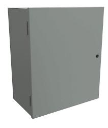
Hammond enclosure, NEMA 1, 24 x 20 x 12in (HxWxD), wall mount, carbon steel, ANSI 61 gray, powder coat finish, single-door, 1/4-turn semi-flush latch.
