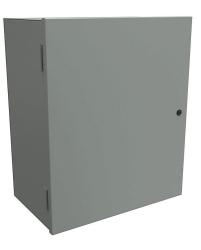
Hammond enclosure, NEMA 1, 24 x 20 x 12in (HxWxD), wall mount, carbon steel, ANSI 61 gray, powder coat finish, single-door, 1/4-turn semi-flush latch.
