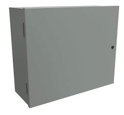
Hammond enclosure, NEMA 1, 20 x 24 x 9in (HxWxD), wall mount, carbon steel, ANSI 61 gray, powder coat finish, singledoor, 1/4-turn semi-flush latch.
