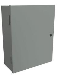
Hammond enclosure, NEMA 1, 20 x 16 x 7in (HxWxD), wall mount, carbon steel, ANSI 61 gray, powder coat finish, single-door, 1/4-turn semi-flush latch.
