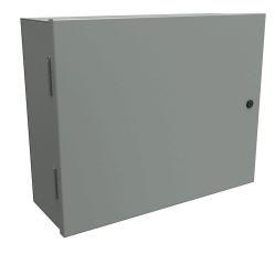
Hammond enclosure, NEMA 1, 16 x 20 x 7in (HxWxD), wall mount, carbon steel, ANSI 61 gray, powder coat finish, single-door, 1/4-turn semi-flush latch.
