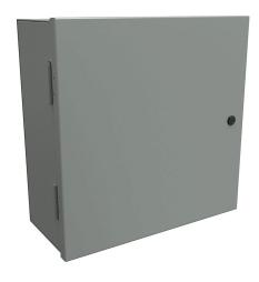
Hammond enclosure, NEMA 1, 16 x 16 x 7in (HxWxD), wall mount, carbon steel, ANSI 61 gray, powder coat finish, single-door, 1/4-turn semi-flush latch.
