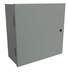
Hammond enclosure, NEMA 1, 16 x 16 x 7in (HxWxD), wall mount, carbon steel, ANSI 61 gray, powder coat finish, single-door, 1/4-turn semi-flush latch.
