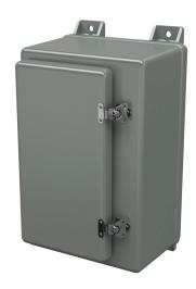
Stahlin N series enclosure, NEMA 1/3/3R/4X/12,  $16 \times 10 \times 7$ in (HxWxD), wall mount, fiberglass reinforced polyester, gray, singledoor, (2) twist-lock latches.
