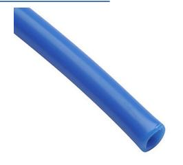
NITRA pneumatic tubing, nylon 12, blue, 1/4in outside diameter, 0.180in inside diameter, 100ft package.
