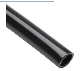
NITRA pneumatic tubing, nylon 12, black, 12mm outside diameter, 10mm inside diameter, 100ft package.
