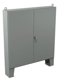
Wiegmann enclosure, NEMA 12, 72 x 72 x 12in (HxWxD), floor mount, carbon steel, ANSI 61 gray, powder coat finish, doubledoor, 3-point keylocking/padlocking combo handle.
