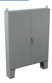
Wiegmann enclosure, NEMA 12, 72 x 60 x 10in (HxWxD), floor mount, carbon steel, ANSI 61 gray, powder coat finish, doubledoor, 3-point keylocking/padlocking combo handle.
