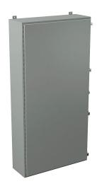
Wiegmann enclosure, NEMA 12/13, 72 x 36 x 12in (HxWxD), wall mount, carbon steel, ANSI 61 gray, powder coat finish, singledoor, (4) plated steel clamps, padlock hasp and staple.
