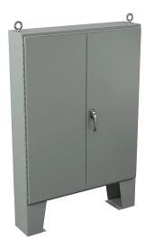
Wiegmann enclosure, NEMA 12, 60 x 48 x 10in (HxWxD), floor mount, carbon steel, ANSI 61 gray, powder coat finish, doubledoor, 3-point keylocking/padlocking combo handle.
