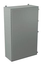
Wiegmann enclosure, NEMA 12/13, 60 x 36 x 16in (HxWxD), wall mount, carbon steel, ANSI 61 gray, powder coat finish, singledoor, (3) plated steel clamps, padlock hasp and staple.
