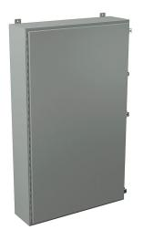
Wiegmann enclosure, NEMA 12/13, 60 x 36 x 10in (HxWxD), wall mount, carbon steel, ANSI 61 gray, powder coat finish, single-door, (3) plated steel clamps, padlock hasp and staple.
