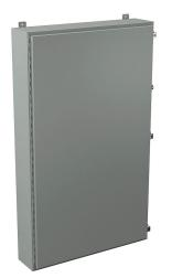
Wiegmann enclosure, NEMA 12/13, 60 x 36 x 8in (HxWxD), wall mount, carbon steel, ANSI 61 gray, powder coat finish, single-door, (3) plated steel clamps, padlock hasp and staple.
