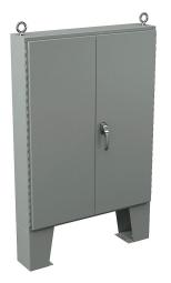
Wiegmann enclosure, NEMA 12, 54 x 42 x 8in (HxWxD), floor mount, carbon steel, ANSI 61 gray, powder coat finish, doubledoor, 3-point keylocking/padlocking combo handle.
