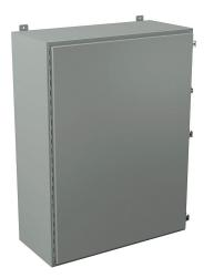
Wiegmann enclosure, NEMA 12/13, 48 x 36 x 16in (HxWxD), wall mount, carbon steel, ANSI 61 gray, powder coat finish, single-door, (3) plated steel clamps, padlock hasp and staple.
