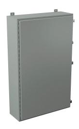
Wiegmann enclosure, NEMA 12/13, 48 x 30 x 10in (HxWxD), wall mount, carbon steel, ANSI 61 gray, powder coat finish, single-door, (3) plated steel clamps, padlock hasp and staple.
