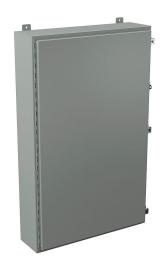
Wiegmann enclosure, NEMA 12/13, 48 x 30 x 8in (HxWxD), wall mount, carbon steel, ANSI 61 gray, powder coat finish, singledoor, (3) plated steel clamps, padlock hasp and staple.
