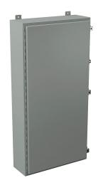
Wiegmann enclosure, NEMA 12/13, 48 x 24 x 8in (HxWxD), wall mount, carbon steel, ANSI 61 gray, powder coat finish, singledoor, (3) plated steel clamps, padlock hasp and staple.
