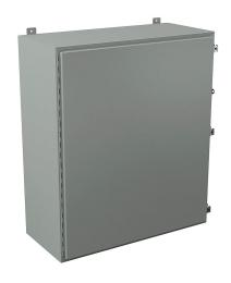
Wiegmann enclosure, NEMA 12/13, 42 x 36 x 16in (HxWxD), wall mount, carbon steel, ANSI 61 gray, powder coat finish, singledoor, (3) plated steel clamps, padlock hasp and staple.
