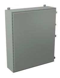
Wiegmann enclosure, NEMA 12/13, 42 x 36 x 10in (HxWxD), wall mount, carbon steel, ANSI 61 gray, powder coat finish, singledoor, (3) plated steel clamps, padlock hasp and staple.
