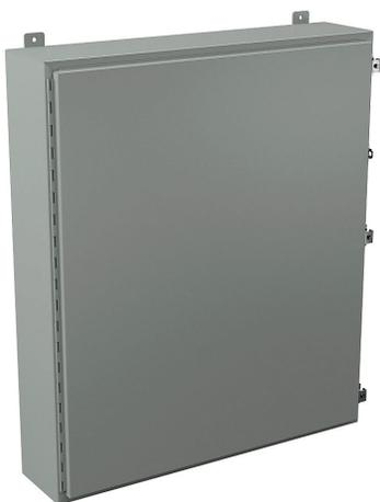
Wiegmann enclosure, NEMA 12/13, 42 x 36 x 8in (HxWxD), wall mount, carbon steel, ANSI 61 gray, powder coat finish, single-door, (3) plated steel clamps, padlock hasp and staple.
