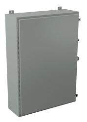
Wiegmann enclosure, NEMA 12/13,  $42 \times 30 \times 10$  in (HxWxD), wall mount, carbon steel, ANSI 61 gray, powder coat finish, single-door, (3) plated steel clamps, padlock hasp and staple.
