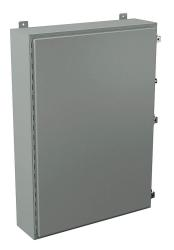
Wiegmann enclosure, NEMA 12/13,  $42 \times 30 \times 8$  in (HxWxD), wall mount, carbon steel, ANSI 61 gray, powder coat finish, single-door, (3) plated steel clamps, padlock hasp and staple.
