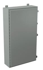
Wiegmann enclosure, NEMA 12/13, 42 x 24 x 8in (HxWxD), wall mount, carbon steel, ANSI 61 gray, powder coat finish, single-door, (3) plated steel clamps, padlock hasp and staple.
