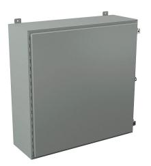
Wiegmann enclosure, NEMA 12/13, 36 x 36 x 12in (HxWxD), wall mount, carbon steel, ANSI 61 gray, powder coat finish, single-door, (2) plated steel clamps, padlock hasp and staple.
