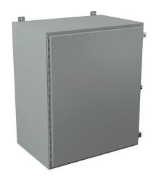
Wiegmann enclosure, NEMA 12/13, 36 x 30 x 20in (HxWxD), wall mount, carbon steel, ANSI 61 gray, powder coat finish, singledoor, (2) plated steel clamps, padlock hasp and staple.
