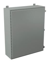
Wiegmann enclosure, NEMA 12/13, 36 x 30 x 10in (HxWxD), wall mount, carbon steel, ANSI 61 gray, powder coat finish, singledoor, (2) plated steel clamps, padlock hasp and staple.
