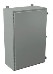
Wiegmann enclosure, NEMA 12/13,  $36 \times 24 \times 12$  in (HxWxD), wall mount, carbon steel, ANSI 61 gray, powder coat finish, single-door, (2) plated steel clamps, padlock hasp and staple.
